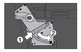
■ Press the light-coloured button under the handle of the brew unit ① and whilst doing so turn the handle in the direction of the arrow ②.
